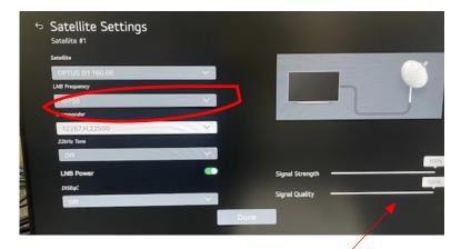
NB- Signal with 10750 LNB Frequency
